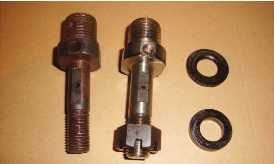
Photo 3: Old and new pins and the two washers.
