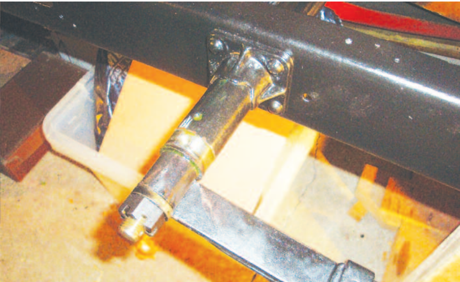
Photo 6: New hanger pin, washers and spring trial assembly.
