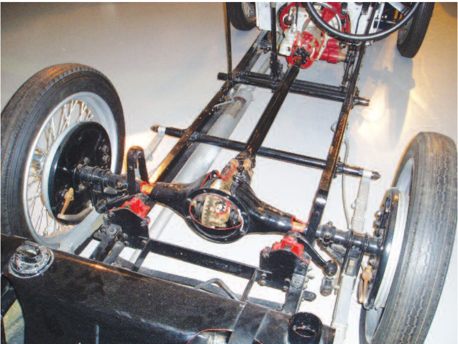
Photo 1: General view of the PA chassis at Gaydon showing the rear axle and springs.
