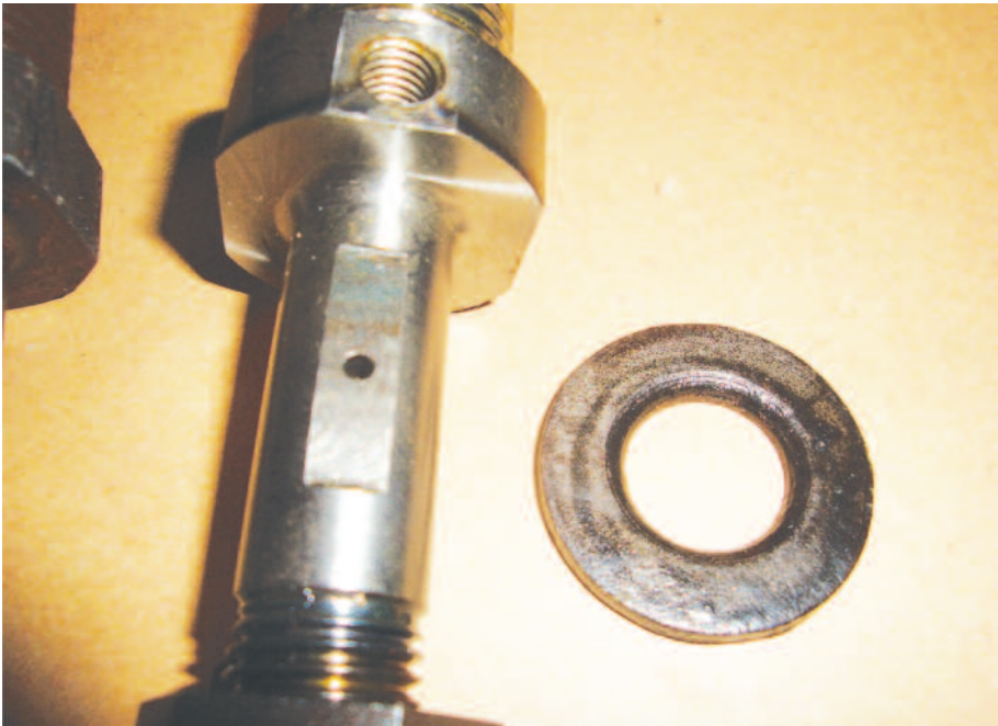
Photo 4: Close up of chamfered face of washer.
